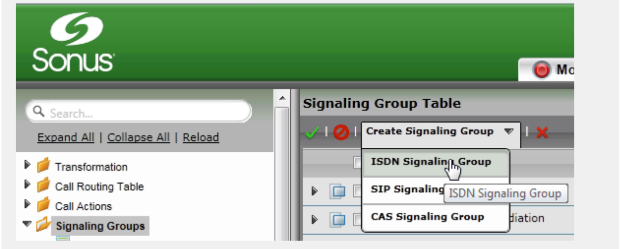
Figure 4: Create ISDN Signaling Group
